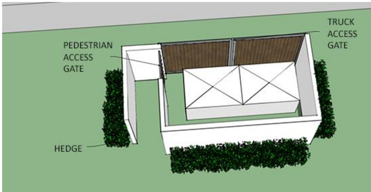
*Example of a refuse storage container that is screened by an opaque wall and incorporates landscaping on sides that face adjacent properties.*
